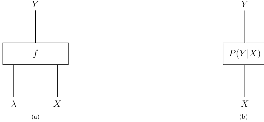
Figure 7: A deterministic structural equation model (SEM) and a classical probabilistic causal model obtained from it. (a) A very simple deterministic structural equation: Y = f(\lambda, X) . (b) A very simple classical channel obtained from this deterministic SEM by averaging over \lambda .
